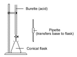
Titrations are used when an acid reacts with an alkali to produce a salt. A pipette is used to measure an exact volume e.g. 25 cm<sup>3</sup> of an alkaline reactant. The second reactant (acid) is poured into a burette through a funnel.
