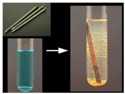
Copper Chloride will change colour from blue to orange (iron (III) chloride). As copper is formed, a brown solid will be formed around the silver iron metal.
